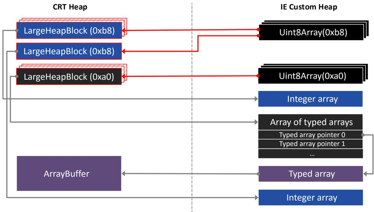
On the left side you can see all the memory which is allocated on the CRT heap while on the right side all IE custom heap allocations are shown. As can be seen, `LargeHeapBlock` objects as well as the data buffers of typed arrays are allocated on the CRT heap. Arrays as well as the typed arrays are allocated on the IE custom heap.
